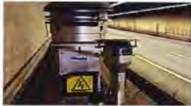
The sampling equipment used to measure PM10 emissions in the Hatfield Tunnel, Hertfordshire (photo: Samantha Lawrence)
