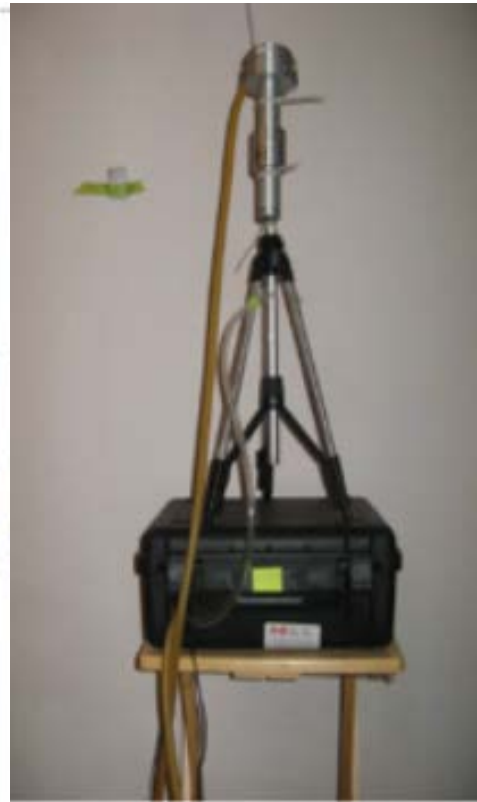
PM 2.5um Harvard Impactor set-up in room
