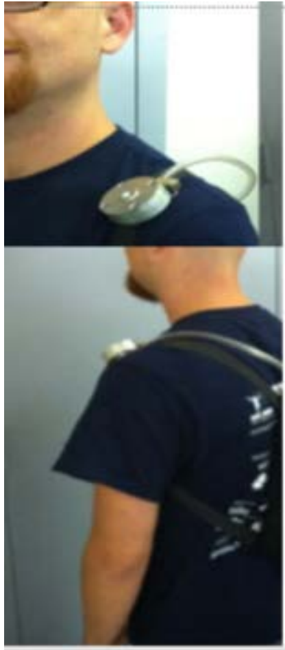
PM 2.5um Harvard Impactor set-up in room
